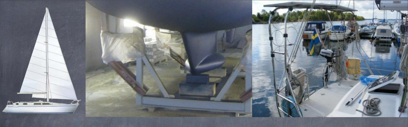
2011 Lucca got a protective Epoxy-treatment (WREDE / Germany) and new Antifouling.. The rusty CQR Anchor was replaced with a 20kg MANSON SUPREME.
